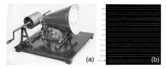
Figure 2.1 - Karl Rudolph Koenig's reconstruction of Scott de Martinville's Phonautograph as photographed; whose form has semblance to gramophone – only that it is working to capture sound rather than emit it (a). Depictions of the recordings of phonautograph, demonstrating the same principles used in vinyl records (b). [Images taken from *Smithsonian's Albert H. Small Documents Gallery* at americanhistory.si.edu]
