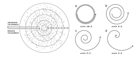
Figure 6.14 - A diagram visualising how the input for changing Artefact's tolerance affects its range and the curvature of the navigation path. The distance between each revolution step (a-b-c-d on right hand side) from a to b increases logarithmically as the tolerance increases to cover the increased range (on left hand side).
