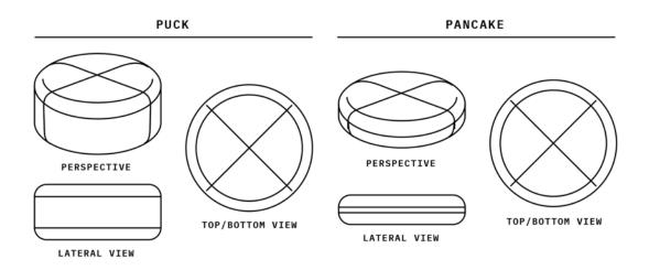
Figure 6.24 - Perspective, lateral, and top/bottom views of puck-shaped and pancakeshaped filleted cylindrical slabs.
