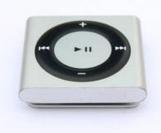
Figure 2.8 - iPod Shuffle is an artefact with a small form factor, which relies on music sequence and shuffling (hence the name) to navigate through a music archive without utilising visual mode. [Photo by Glen Carrie on Unsplash]
