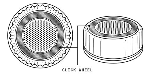
Figure 6.31 - The click wheel encircling the screen is used for adjusting secondary controls that don't have effect on directionality, temporality, and tolerance of music playback.
