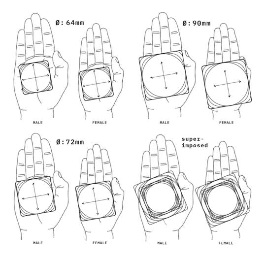
Figure 6.22 - A diagram visualising how primitive shapes between circle and square with diameters of 64, 72, and 90 millimetres compare to each other.
