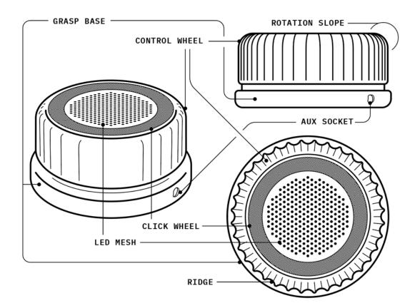
Figure 6.32 - Conclusive conceptual design for visualising how the interactivity features affect the enclosure and outer components.
