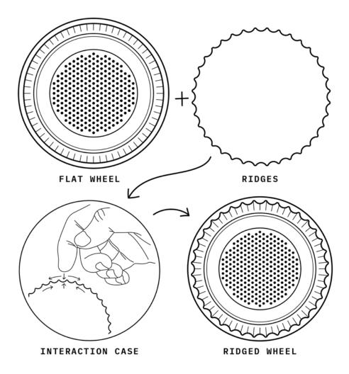
Figure 6.29 - Visualising the inclusion of ridges onto the wheel for supporting the omnidirectional rotation atop the user's fingers -no, the ridges don't represent servations.
