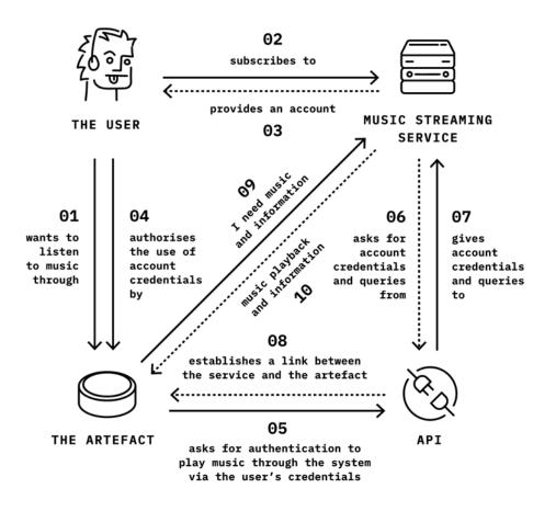
Figure 6.17 - Process of authenticating the Artefact with access to a music streaming service for music playback and meta data.
